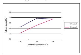
As the conditioning time and temperature was increased, the pellet durability increased (as expressed by a Holmen Durability Index).
