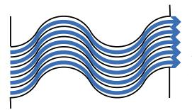
Figure 8. One type of commercial light trap is called variously an "S," "W,""blade" or "vane" trap. This type trap, if well designed, can block light well without overly restricting airflow.
