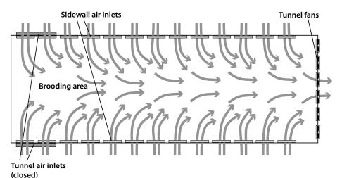
Operating minimum ventilation on a 5-minute timer minimizes temperature and RH extremes and provides a better rearing environment.
