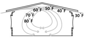
The amount of house heat lost during proper minimum ventilation is insignificant compared with the benefits gained. Even when ammonia is not an issue (as with new litter and/or litter treatments), failure to provide adequate fresh air and to break up in-house air stratification can be very costly in terms of bird health and growth.
