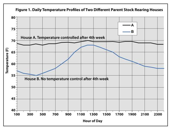
Benefits of in-house environmental control are shown in these two graphs, depicting otherwise identical houses and flocks. In House A, with supplemental heat provided after the 4th week to keep house temperature between 68° F and 70° F, birds required much less feed (Etotal-A vs Etotal-B below). To maintain desired target weights, birds in House B with no temperature control required 1.67 lb more feed per pullet, for a total additional feed cost of \$1,612.
