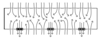
The three basic ventilation modes use different types and placements of fans and air inlets to create the air exchange rates and airflow patterns needed.
